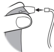
Reconnect the thin tube to the hearing instrument.
