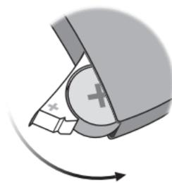
Close the battery drawer. The instrument will play a jingle through the ear piece. Hold the earpiece close to your ear to hear the jingle.
