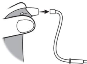
Pull the thin tube out of the hearing instrument
